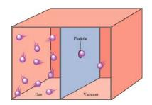
The rates of effusion of two gases are inversely proportional to the square roots of their molar masses at the same temperature and pressure.
