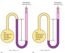
The **manometer**—a device for measuring the pressure of a gas in a container. The pressure of the gas is given by h [the difference in mercury levels] in units of torr (equivalent to mm Hg).
