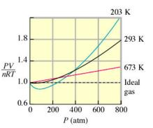
This graph is just for nitrogen gas. Note that although nonideal behavior is evident at each temperature, the deviations are smaller at the higher Ts.
